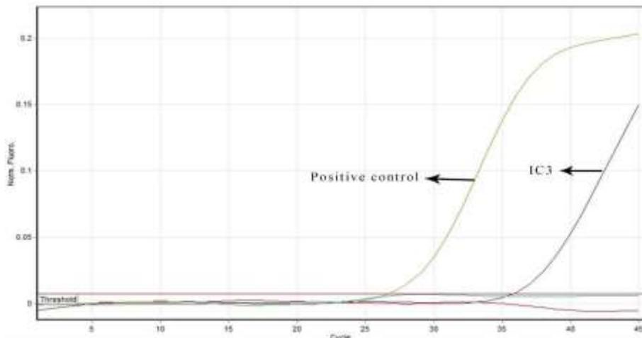
**Fig. 3.** Amplification plot of E gene on ROX channel of Rotor-Gene 6000 instrument on insect specimens using multiplex one-step qPCR along with positive and negative control
